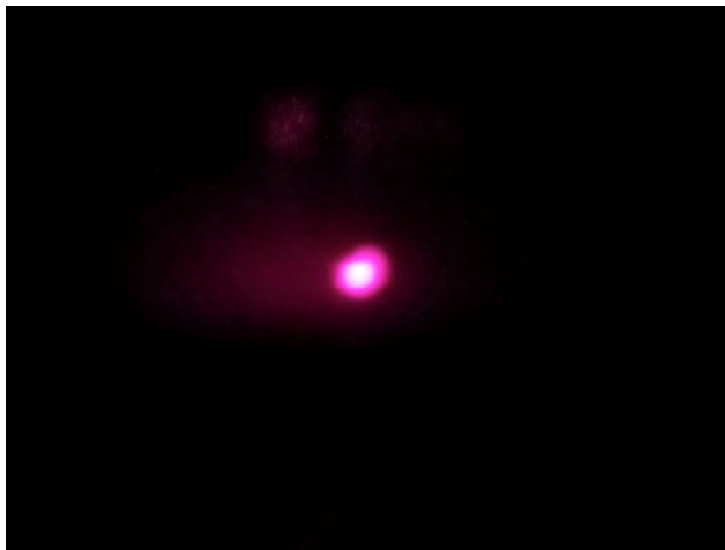
A view of the trapped atoms in the vacuum chamber. Approximately ten million atoms are trapped by a combination of six intersecting red laser beams and a magnetic field. The red ball of atoms at a temperature of a few hundred microkelvin is approximately 0.5 mm across.
