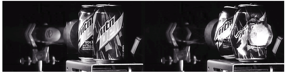
Figure 1. Ping-pong balls exit the cannon at about 300 meters per second (or 670 miles/hour). The pictures above show the ball about to exit the cannon (left) and after taking the “short way around” two pop cans. Check out the full video at 25,000 frames per second to see the full sequence “at a snail’s pace.”
